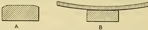
Fig. 51 —(A) A file held in the manner pictured in Fig. 48 will cut the corners of the work off as shown. (B) How a file bends when held in the manner pictured in Fig. 50
